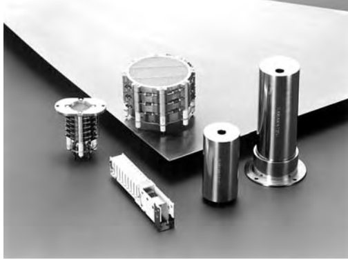
Figure 12-1: Electron multiplier tubes
