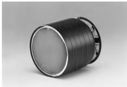
Figure 9-26: Grid type dynode photomultiplier tube
