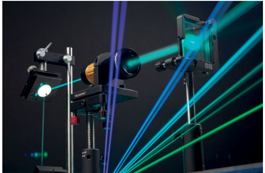
FIG. 2: An example of a high energy laser setup where LDT considerations of the optics is crucial.
