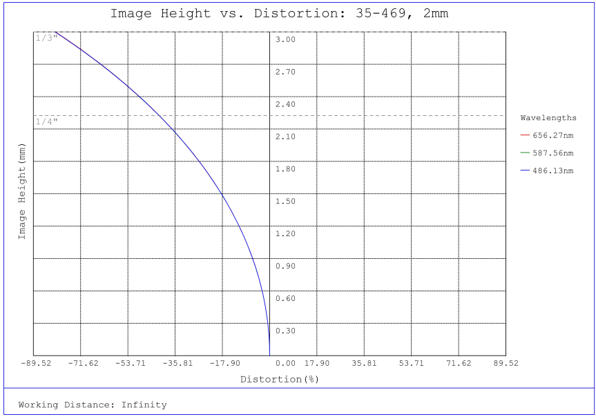
#35-469, 2mm FL f/2.5 IR-Cut Rugged Blue Series M12 Lens, Distortion Plot
