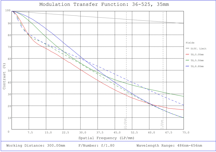
#36-525, 35mm f/1.8, HPr Series Fixed Focal Length Lens, Modulated Transfer Function (MTF) Plot, 300mm Working Distance, f1.8
