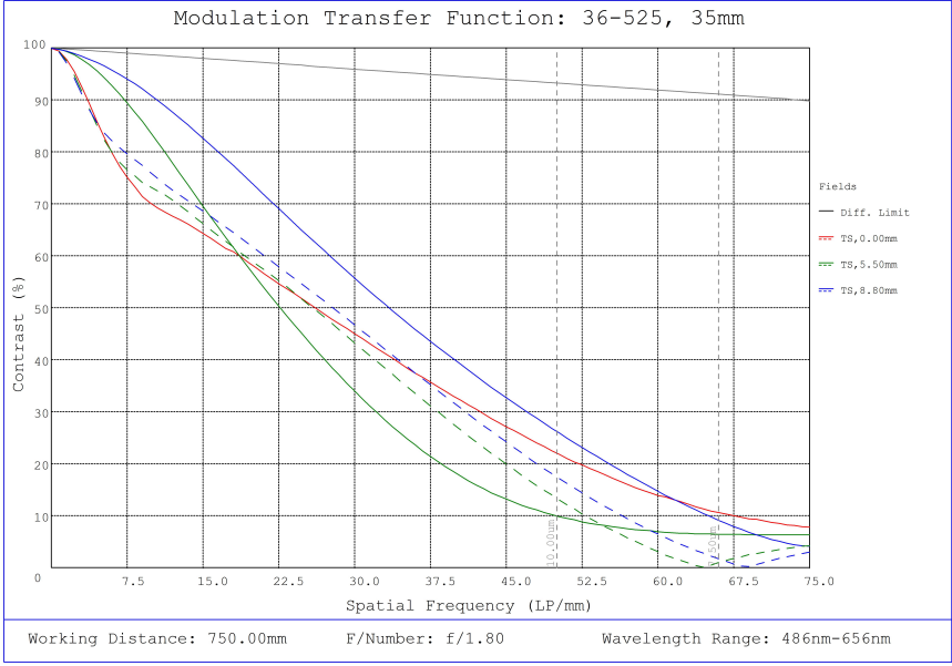
#36-525, 35mm f/1.8, HPr Series Fixed Focal Length Lens, Modulated Transfer Function (MTF) Plot, 750mm Working Distance, f1.8
